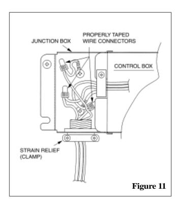
Connect the power line to the black, white and ground wires found in the junction box using three wire connectors. CAUTION - Connect black wire to black wire, white wire to white wire and ground wire to ground wire. (green to bare copper) Using UL approved electrician's tape, secure the wire connectors in a workmanlike manner. See Figure 11.
