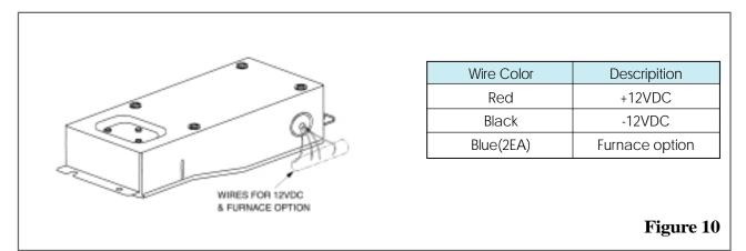
Remove the electric control box cover. (2 screws) Take the supply wire and slide it into the side of the junction box through the strain relief that is provided.
