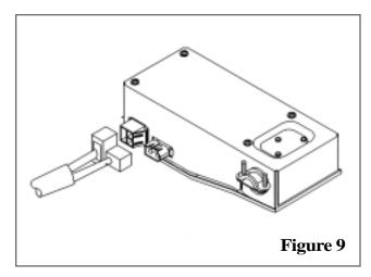
Connect the 12 VDC lines to the black and the red wires using UL approved electrician's tape. One supply lead must be +12 VDC and red in color. The second supply lead must be -12 VDC and black in color. CAUTION! - Connect red wire to +12 VDC wire, black wire to -12 VDC wire. If a furnace is also to be operated, additional wiring (2 blue wires) will need to be routed. See Figure 10.
