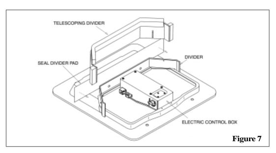
Using the four bolts provided, secure the ceiling assembly frame to the roof top unit. The four mounting bolts are to be applied up through the bottom of the ceiling assembly frame and into the bottom of the roof top unit.
